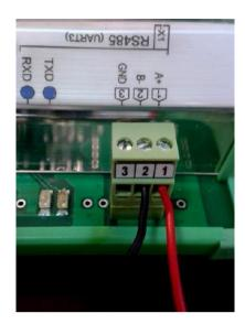
Connecting Modbus meter/device to the MX-9
