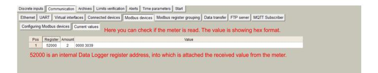
Step 5: Click on **Communication** tab - > **Data transfer** -> **Common parameters**. In this tab are described meter values, formats, headers and dimensions, which will be archived and sent to the FTP. Only archived values can be sent to FTP.
