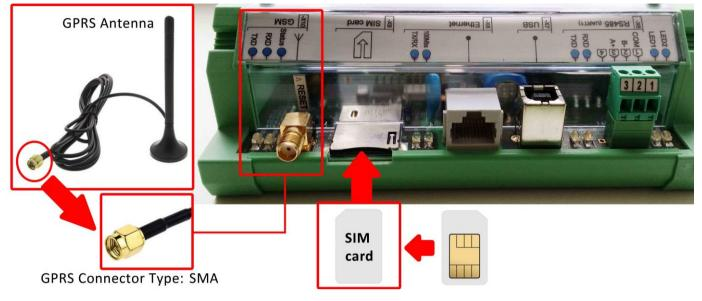
Check GPRS antenna is properly connected to the device. Insert SIM card.
