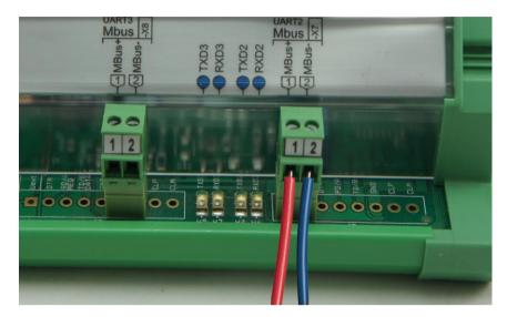
Connecting the M-Bus meter/device to the MX-9 M-Bus interface.
