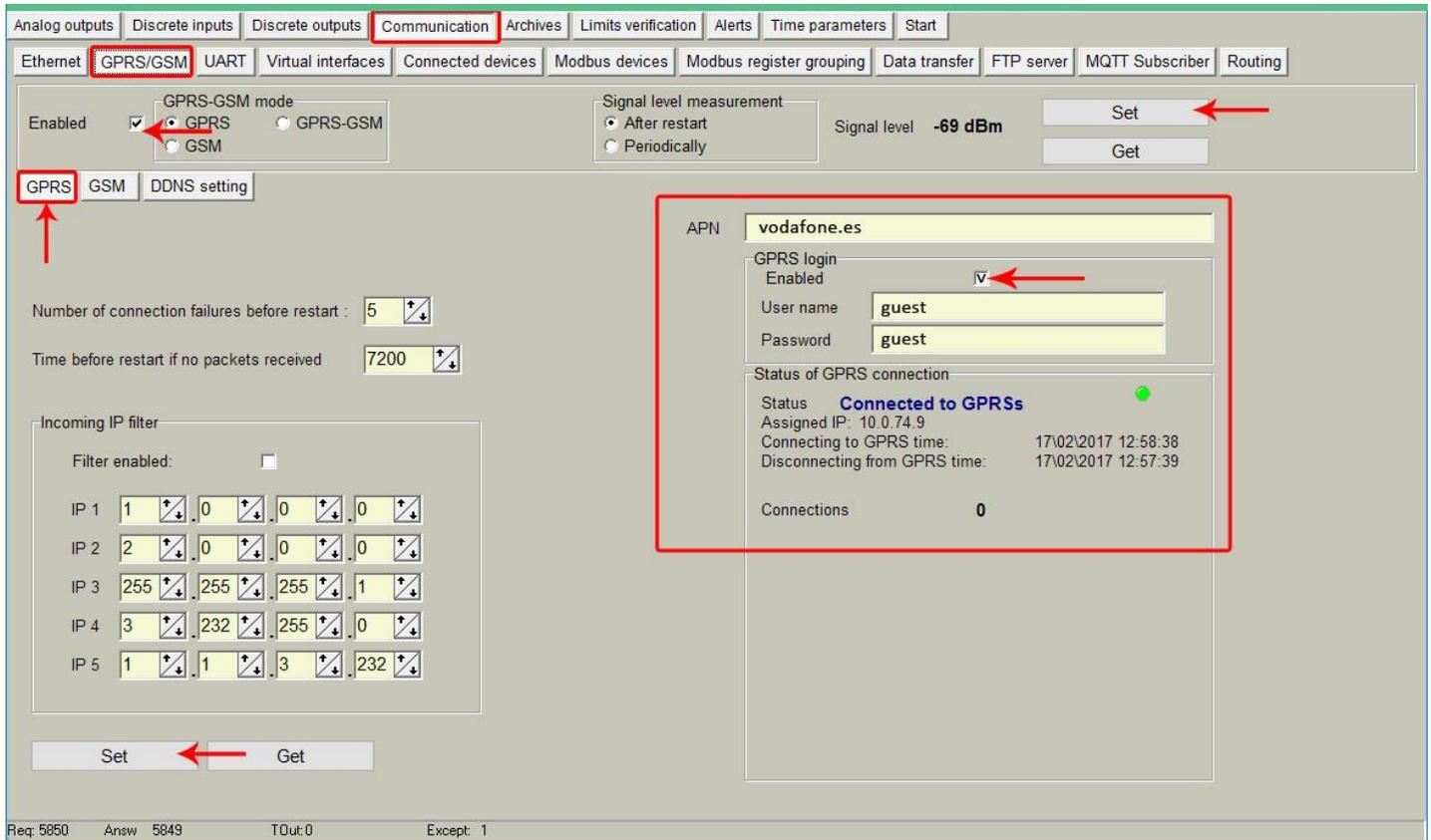
**Pic 14. GPRS Tab. Enabling communication**
