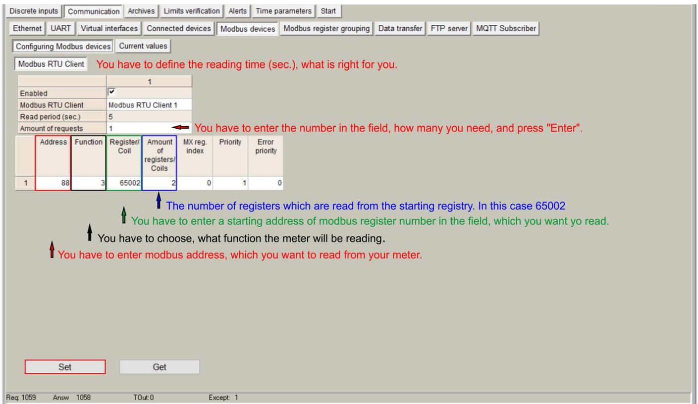
Step 4: Click on **Communication tab - > Modbus devices -> Current values**. In this tab you see if the Modbus meter / device is read. The value is being showed in hex formate. Also there is indication of MX-9 Register adress, where the received modbus value is.
