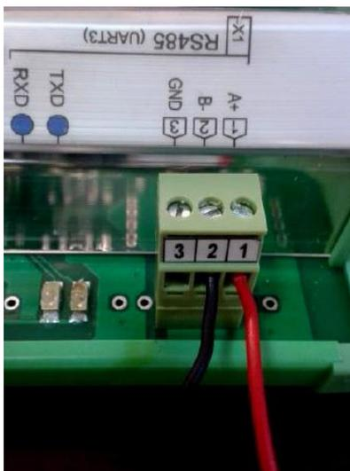
Connecting Modbus meter/device to the MX-9
