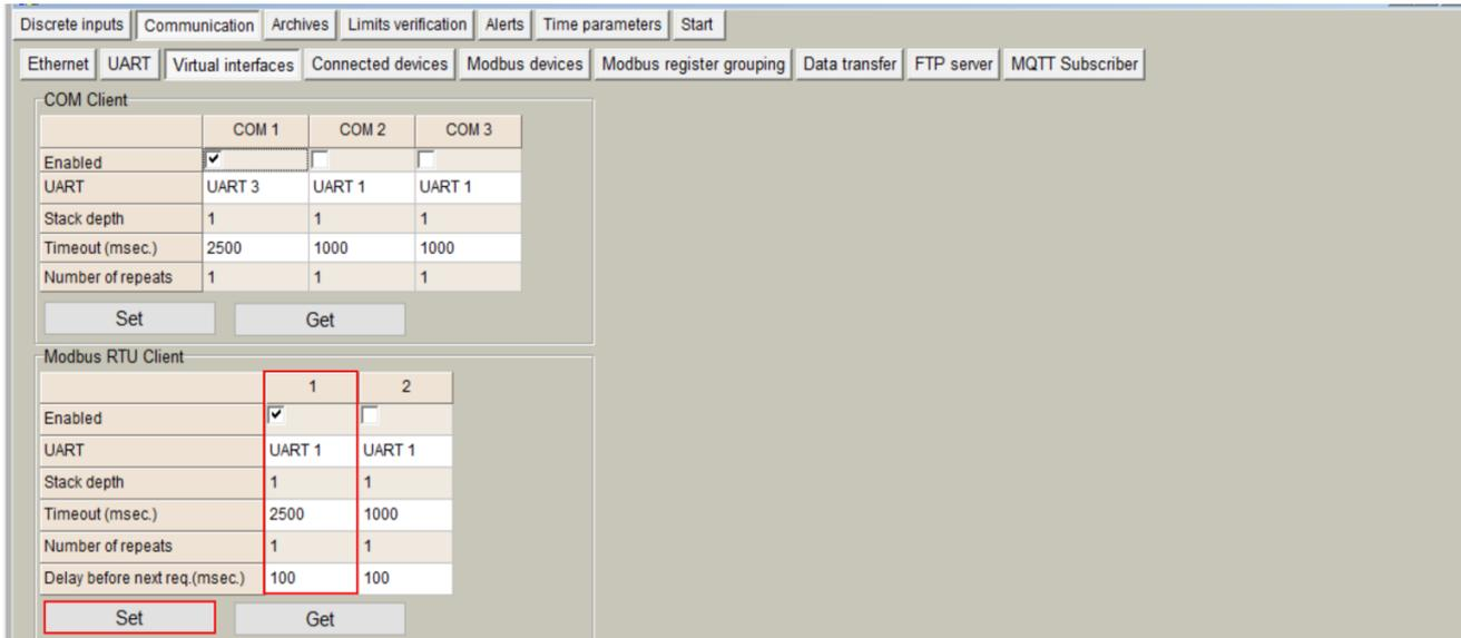
Step 3: Click on **Communication tab** - > **Modbus devices** -> **Configuring Modbus devices** -> **Modbus RTU client**. Define the reading time (sec) by your requirements. Then set the amount of requests, press „Enter“. Also set the Address, Function, Register, and Coils as indicated in the picture above and press „**SET**“.
