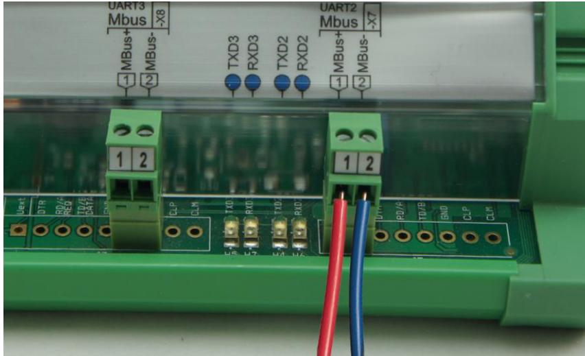
Connecting Modbus meter/device to the MX-9
