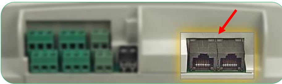
Figure 79: RJ45 connectors for RS485 interface connection (for integrated variant only)
