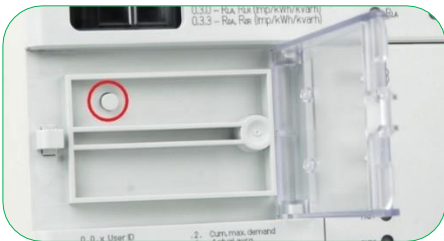
Figure 53: Billing reset button under the transparent window
