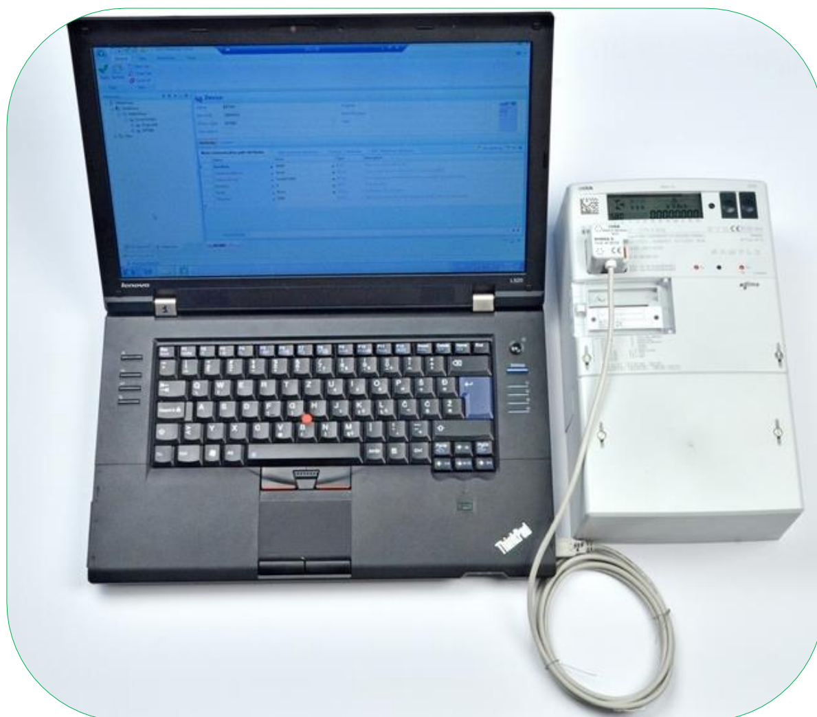
Figure 91: No power reading with SEP2 MeterView – meter supplied by laptop via optical probe
