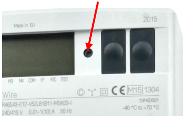
Figure 36: Optical scroll button on the meter
