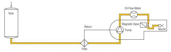
Mounting on suction side of pump (burners)
