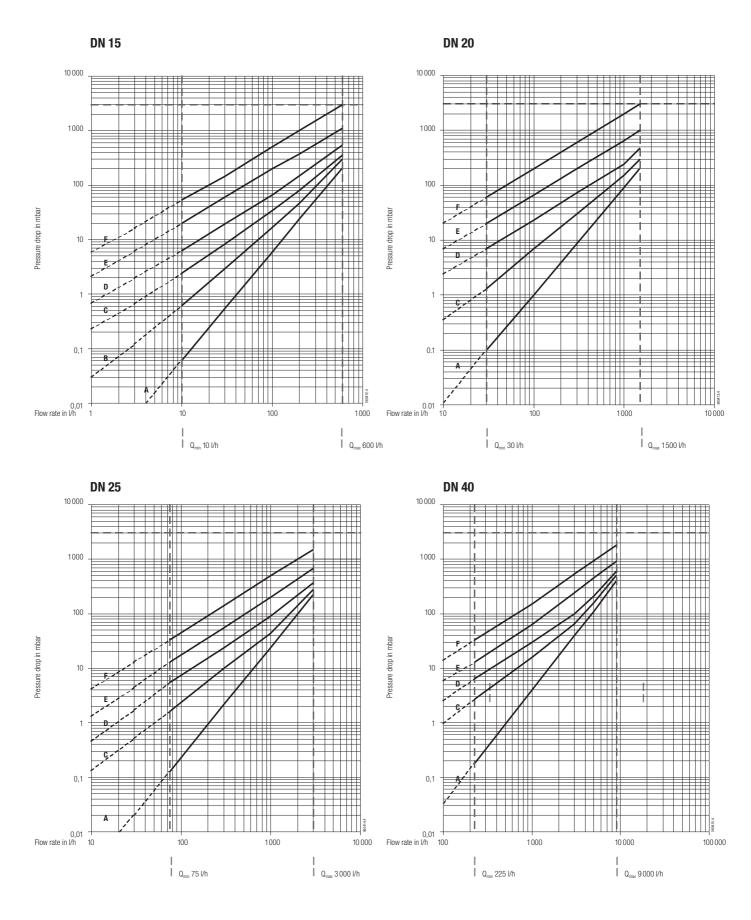
Viscosity diagrams:A = 5 mPa.sC = 50 mPa.sE = 200 mPa.sB = 25 mPa.sD = 100 mPa.sF = 500 mPa.s
